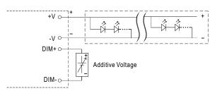
"DO NOT connect "DIM- to -V"
