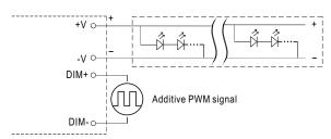
"DO NOT connect "DIM- to -V"
