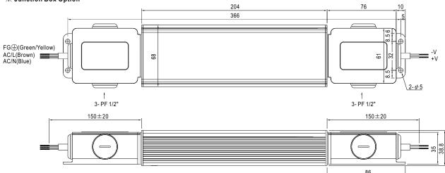
$\bigcirc \ \, {\sf Junction\ box\ option\ is\ available\ for\ A/Blank-Type.\ Please\ contact\ MEAW\ WELL\ for\ details.}$
