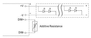
"DO NOT connect "DIM- to -V"
