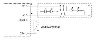
"DO NOT connect "DIM- to -V"
