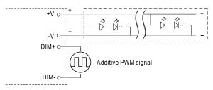
"DO NOT connect "DIM- to -V"
