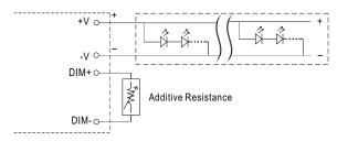
"DO NOT connect "DIM- to -V"
