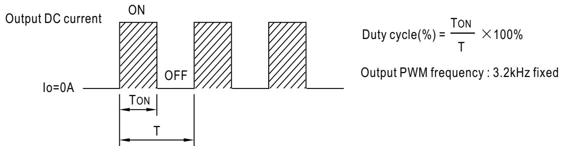
※ Dimming principle for colour temperature dimming and brightness dimming(4 channels output, for DA2Q Type)
